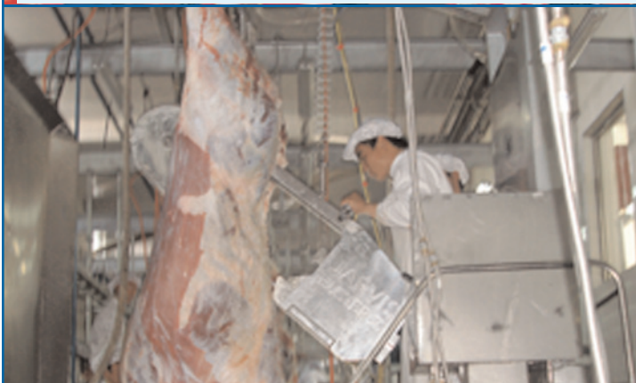
Jarvis tools being used in the new Lianoning Hongda beef processing plant. Above, a Buster V Bandsaw splitting a carcass. Below, a MG-1E Beef Brisket Saw cutting through a brisket section.
