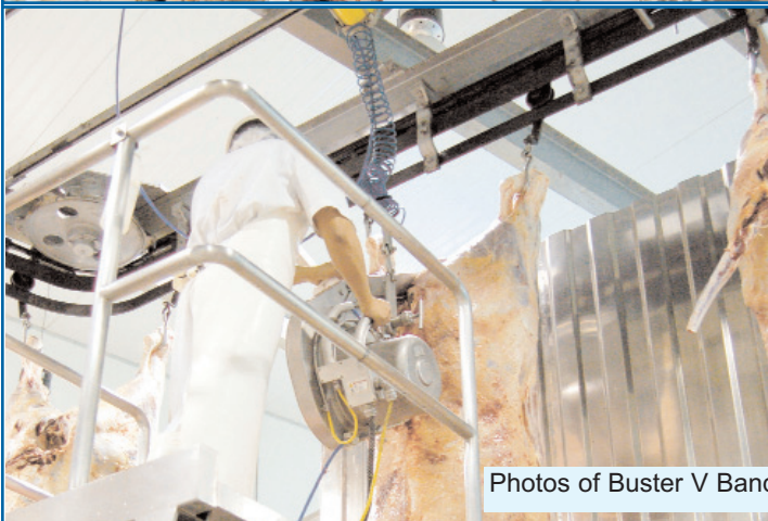
Jarvis' MG-1E Beef Brisket Saw being used for brisket cutting.
