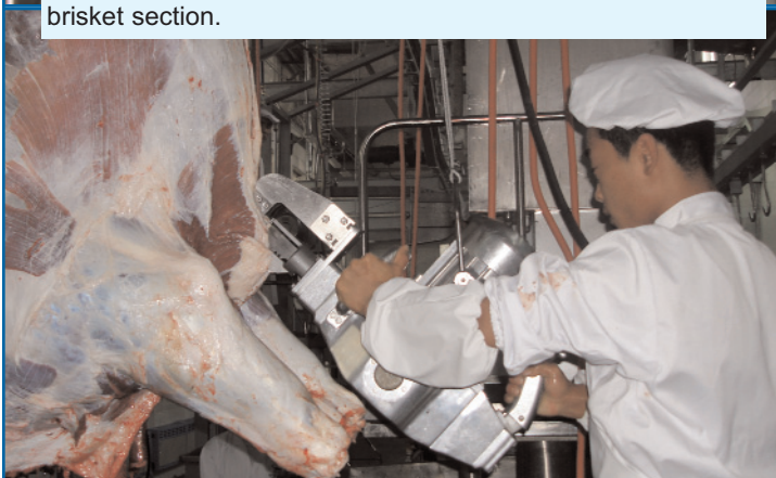
Jarvis tools being used in the new Lianoning Hongda beef processing plant. Above, a Buster V Bandsaw splitting a carcass. Below, a MG-1E Beef Brisket Saw cutting through a brisket section.
