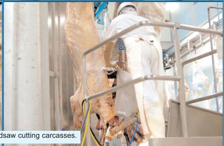
Model 30CL-2 Beef Hock Cutter in action.
